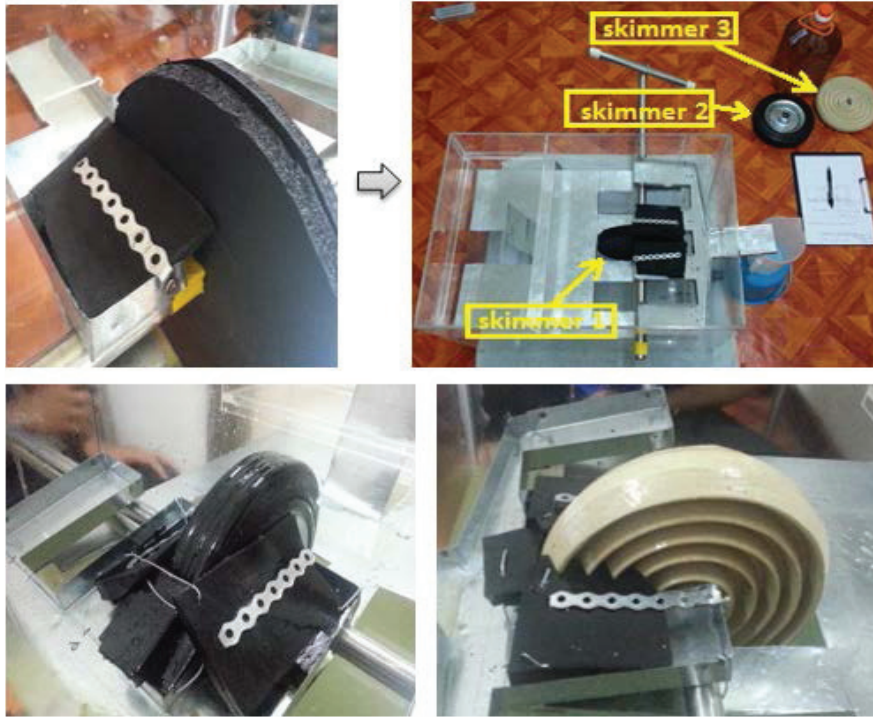
Figure 10. The oil collector and skimmer in position
