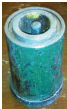
Figure 3 Metal mould used for the briquette
