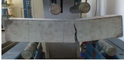
FIGURE 6. Flexure test on concrete beam
