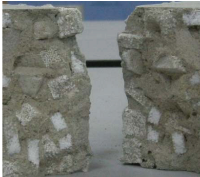
FIGURE 7 Fracture surface under flexural test
