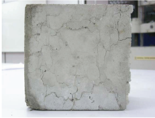
FIGURE 4 Concrete cube under compression test
