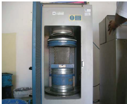
FIGURE 1 Determining compressive strength of polystyrene lightweight aggregate concrete.
