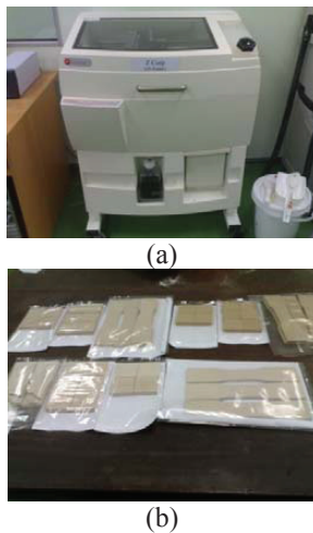
FIGURE 6 (a) Commercial 3D printing machine (b) 3D components produced for mechanical properties test
