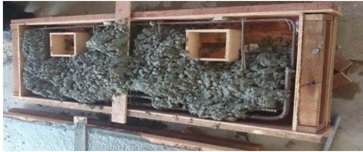
(a) Deep beam with 150 x 150 mm square opening
