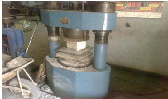
Figure 2. Testing of concrete cubes for compressive strength.
