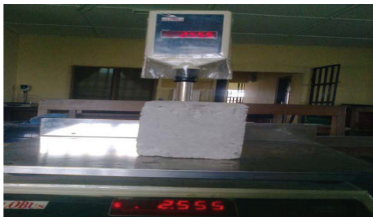
Figure 3. Weighing of specimen before being soaked in water.
