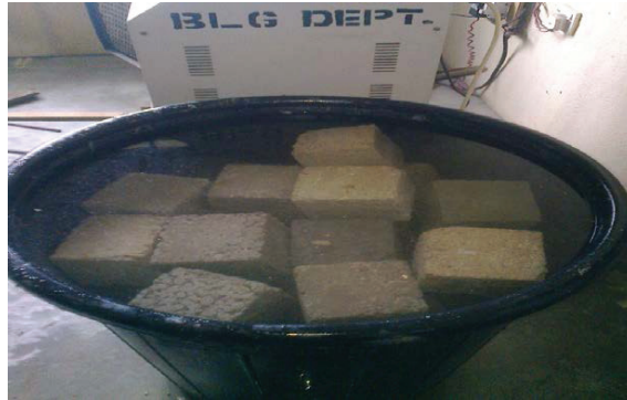
Figure 4. Specimens soaked in water for 24 hours.
