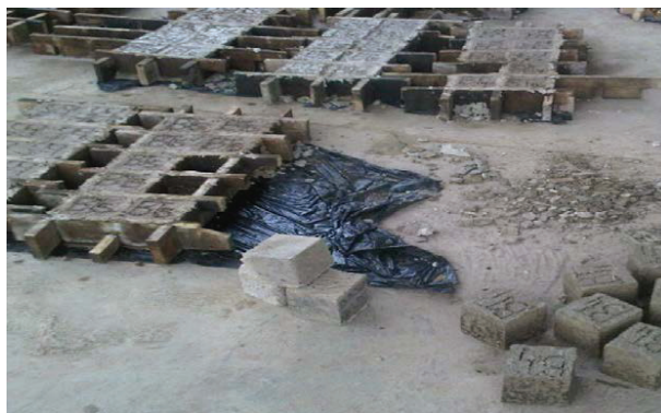
Figure 1. Demoulding of cast concrete cube specimens.
