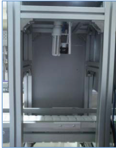
Figure 3. Elements of machine vision and conveyer system.
