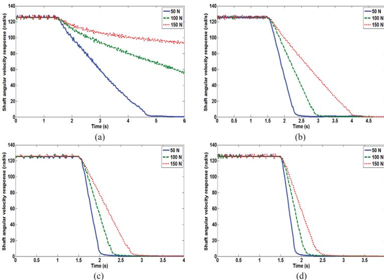
Figure 6. Shaft angular velocity response versus time at various current; (a) 1 A, (b) 2 A, (c) 3 A and (d) 4 A
