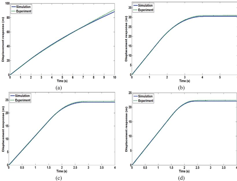
Figure 5. Comparison between model and experimental of load displacement response at several applied current; (a) 1 A, (b) 2 A, (c) 3 A and (d) 4 A
