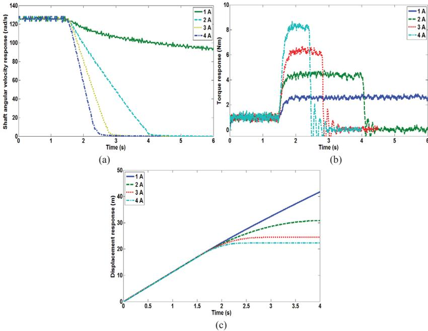
Figure 2. Measured responses at four constant currents; (a) Shaft angular velocity response, (b) Torque response and (c) Load displacement response
