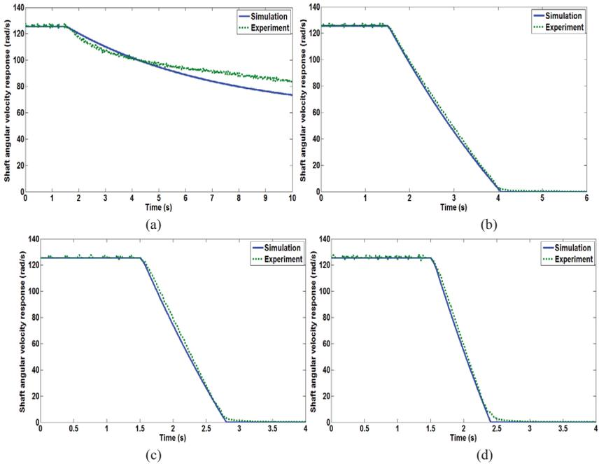
Figure 3. Comparison between model and experimental at several applied current for shaft angular velocity response; (a) 1 A, (b) 2 A, (c) 3 A and (d) 4 A
