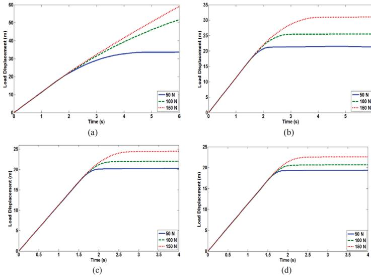
Figure 8. Load displacement response versus time at various current; (a) 1 A, b) 2 A, c) 3 A and d) 4 A
