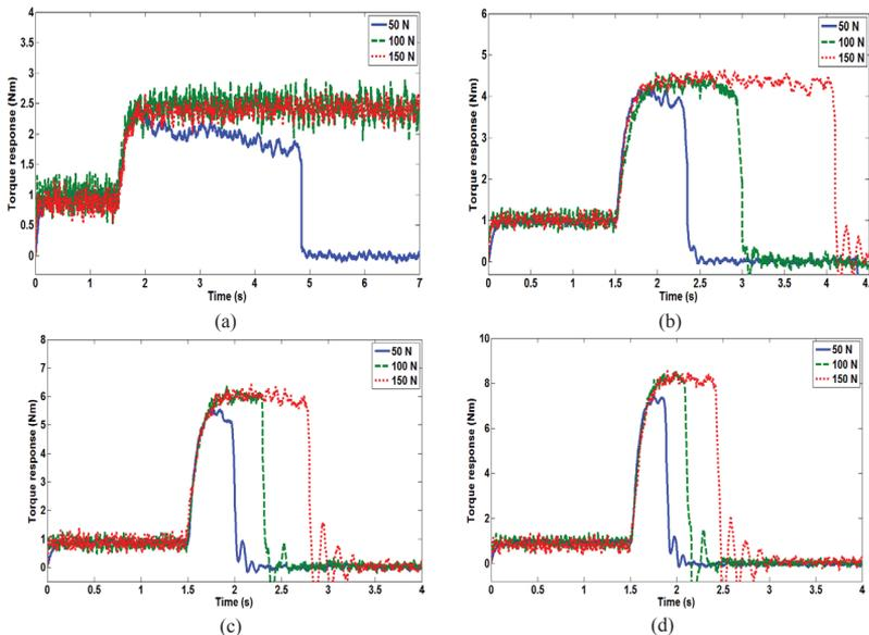
Figure 7. Torque response versus time at various current; (a) 1 A, (b) 2 A, (c) 3 A and (d) 4 A
