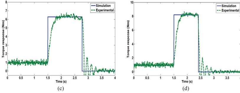
Figure 4. Characteristic of torque response between model and experimental; (a) 1 A, (b) 2 A, (c) 3 A and (d) 4 A
