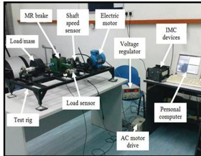
Figure 1. Mechanical assembly of the MR brake test rig
