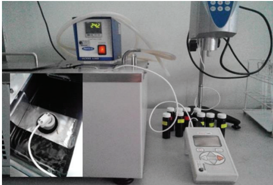
Figure 1. Experimental set-up for thermal conductivity measurement
