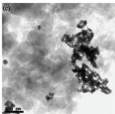
**Figure 2 (c)** TEM images of Pt sols mixing with carbon black to make 5% Pt/C, and (d) Pt/C after re-dispersing (c) in DMAc and then being freeze-dried. The Pt sols preparation conditions: Pt/Nafion = 1/0.34; 90 vol% methanol; T = 85 °C.
