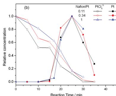
**Figure 1 (b)** The evolution of the normalized concentration of  $\text{PtCl}_6^{2-}$  and Pt nanoparticles based on the maximum absorbance at 261 and 450 nm, respectively, during preparation at 85 °C.
