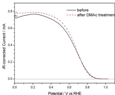
**Figure 4** Effect of DMAc-treatment on the electrochemical reduction of oxygen over Nafion-Pt/C catalysts. The ORR currents were recorded under O<sub>2</sub> at 25 °C, 1600 rpm, and 10 mV s<sup>-1</sup>.
