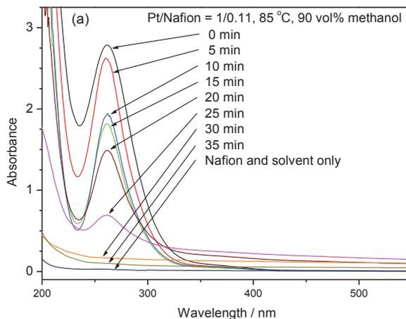
**Figure 1 (a)** UV-visible spectra during the preparation of Nafion-stabilized Pt sols
