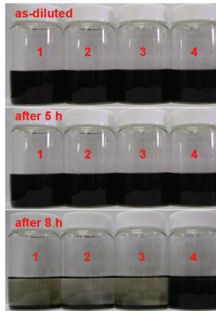
**Figure 3** Effect of diluent solvents on the stability of Pt sol at a 1:1 (vol) ratio at room temperature; 1: methanol; 2: ethanol; 3 n-propanol; 4: DMAc.
