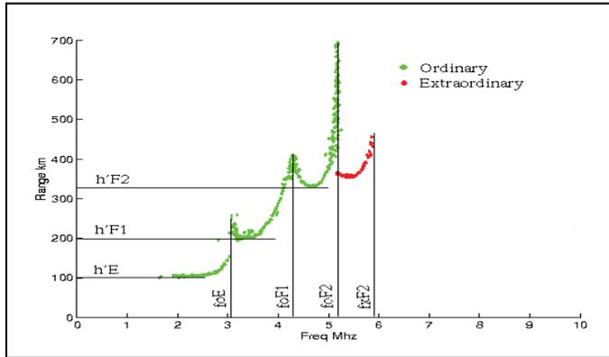
**Figure 2** Sample of an ionogram from ionosonde
