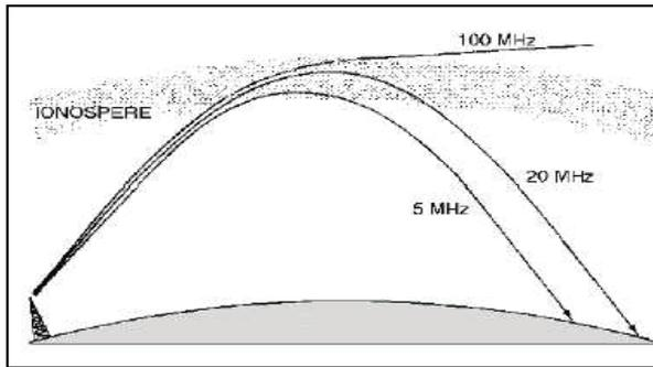
**Figure 1** Illustration of the HF propagation and its relation with  $f_c$  (Pulinet and Boyarchuk, 2004)
