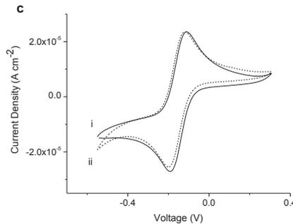
**Figure 4** Cyclic voltammograms of (i) graphene, (ii) oxidized graphene in 1 mM  $\text{Ru}(\text{NH}_3)_6^{2+/3+}$ .
