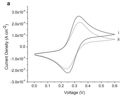
**Figure 3** Cyclic voltammograms of (i) graphene, (ii) oxidized graphene in 1 mM  $\text{Fe}(\text{CN})_4^{3-/4-}$ .
