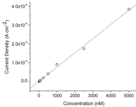
**Figure 8** Calibration curve of NADH oxidation current at oxidized graphene electrode.
