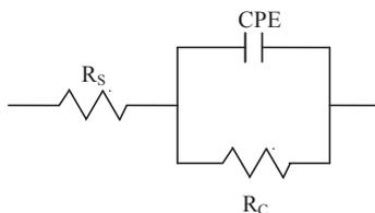
**Schematic 1** Randles equivalent circuit model for graphene and oxidized graphene in 1 mM Fe(CN)<sub>6</sub><sup>3-/4-</sup>.
