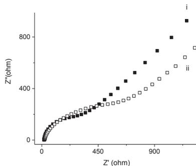
**Figure 5** Nyquist plot of (i) graphene, (ii) oxidized graphene in 1 mM Fe(CN)<sub>6</sub><sup>3-/4-</sup>.
