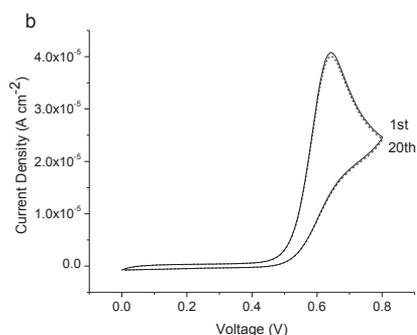
**Figure 7** Cyclic voltammograms for 5  $\mu\text{M}$  NADH in 0.1 M PBS at oxidized graphene electrode at 100  $\text{mV s}^{-1}$ .
