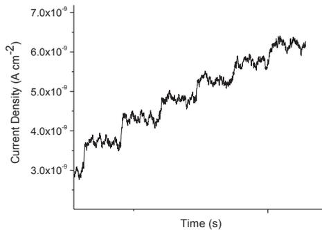
**Figure 9** Amperometry of oxidized graphene electrode towards addition of 10 nM NADH.
