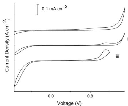
**Figure 1** Electrochemical window of (i) boron-doped diamond, (ii) graphene, (iii) oxidized graphene in 1 M KCl.
