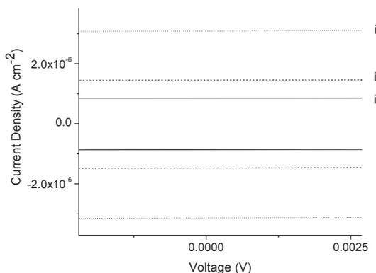
**Figure 2** Background current of (i) boron-doped diamond, (ii) graphene, (iii) oxidized graphene in 1 M KCl.
