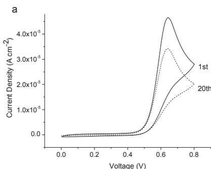
**Figure 6** Cyclic voltammograms for 5  $\mu\text{M}$  NADH in 0.1 M PBS at graphene electrode at 100  $\text{mV s}^{-1}$ .
