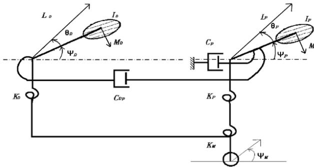
Figure 2 Schematic diagram of wiper system
