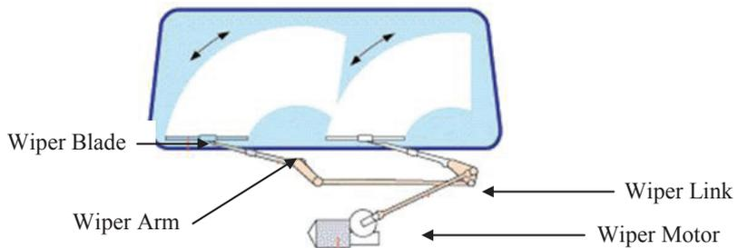
**Figure 1** Wiper system on a windscreen
