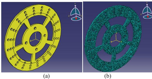
Figure 5 Disc brake rotor (a) before meshing, (b) after meshing
