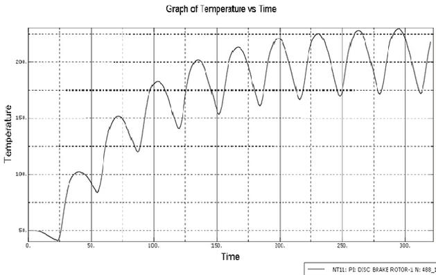
**Figure 6** Surface temperature of the new disc brake rotor for 10<sup>th</sup> cycles of braking
