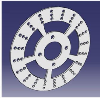
**Figure 2** The 3D model of the new ventilated disc brake rotor design
