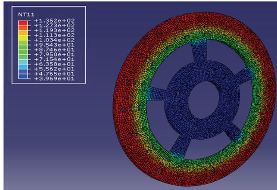
**Figure 7** Temperature distribution of the rotor surface at the end of 1st cycle of braking
