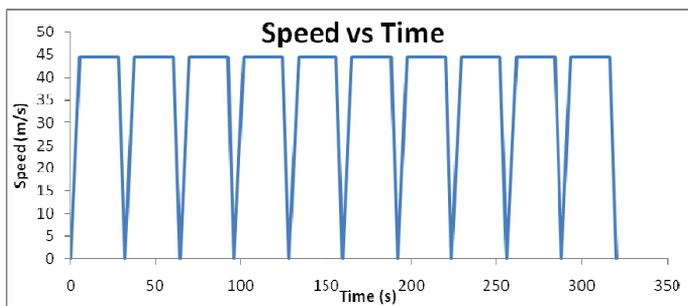
**Figure 3** Speed versus time for 10 cycles of braking
