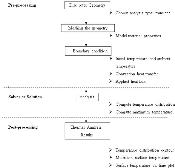
Figure 4 Finite element modeling stages
