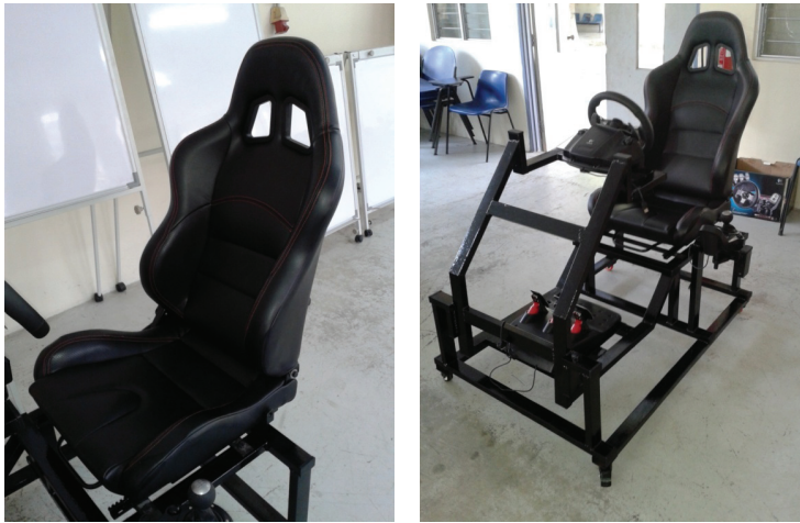
(a) (b) Figure 10. (a) Installation of seat and (b) Complete installation
