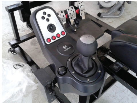
Figure 8. Installation of gear knob
