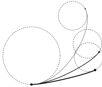
Figure 2. Various designs of C-Transition Curve by using shape control technique (Habib & Sakai, 2009)
