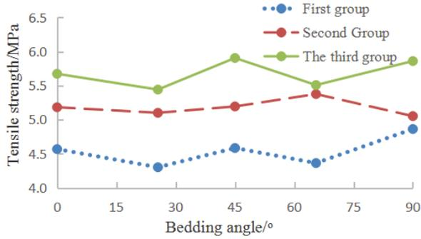
(a) Dynamic tensile strength of coal samples
