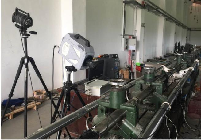
Fig. 2. Test equipment of SHPB
