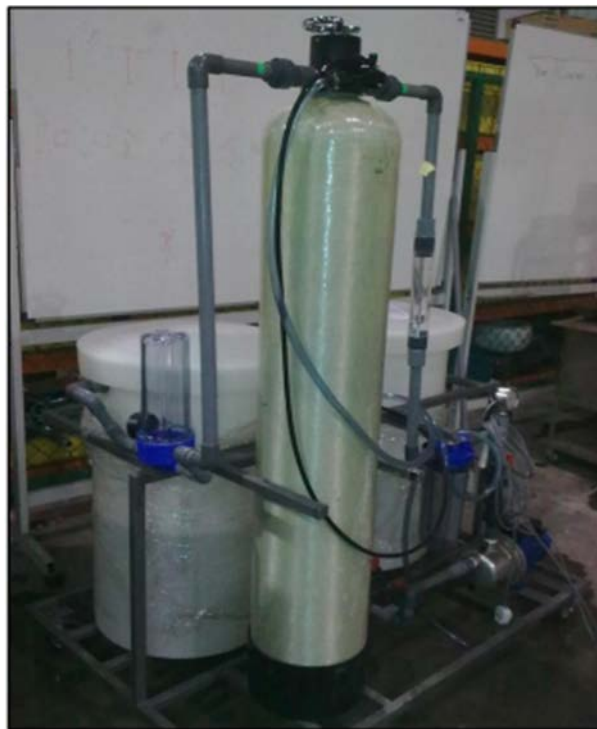
Figure 2. Portable Mercury Removal Rig (PMRR)
