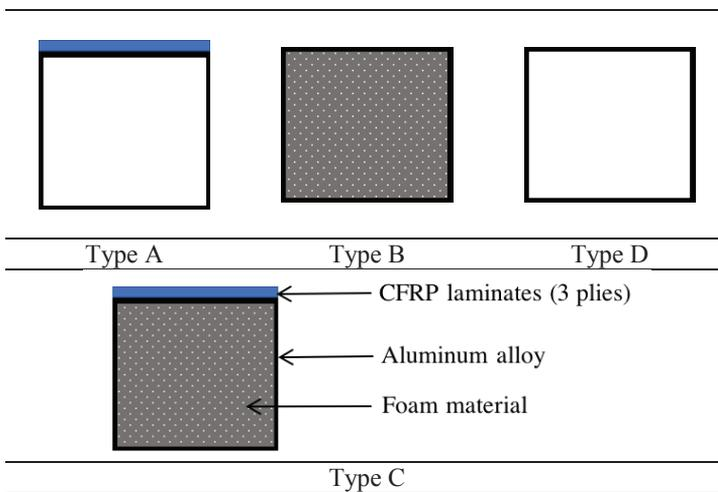
Figure 5. Aluminium Alloy Enhancement (Types A, B, and C), Aluminium Alloy (Type D)
