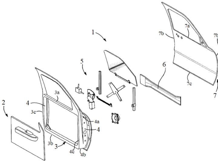
Figure 1. Components In Side Door of a Car (Palazzolo & Hui, 2000)
