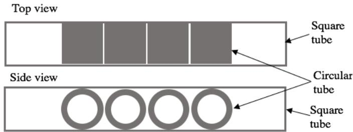
Figure 4. Square Tube Glass Fiber/Epoxy Composites with Circular Glass Fiber/Epoxy Composites Inside (Terada et al., 2009)
