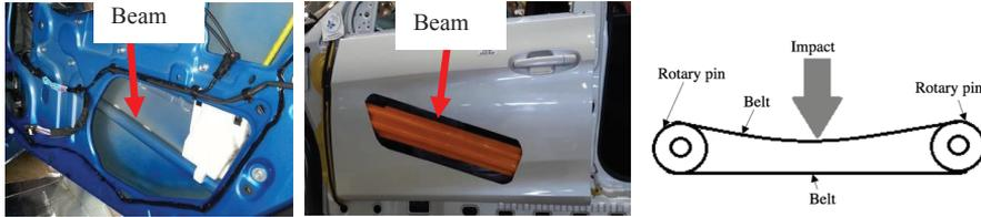
Figure 3. a) Tubular Type, b) Panel Type, c) Belt Type
