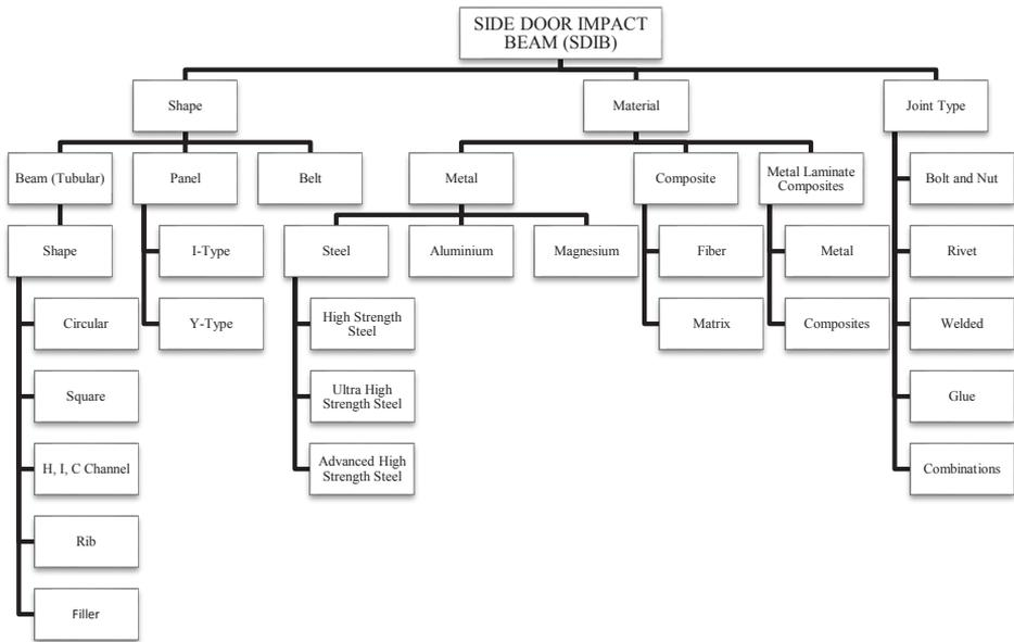
Figure 2. Classification of Side Door Impact Beam
