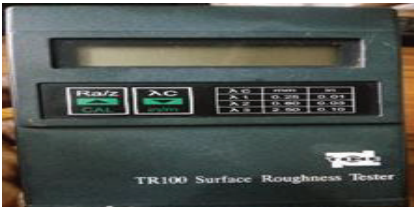
Figure 3: TR100 Ra Tester
