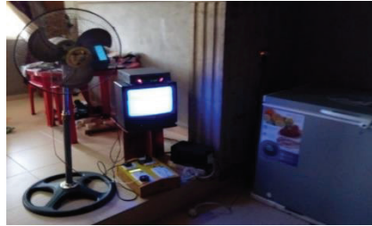
Figure 16: The proposed device with the connected loads when a command *A.1 fanoff# was sent to the proposed HAS
