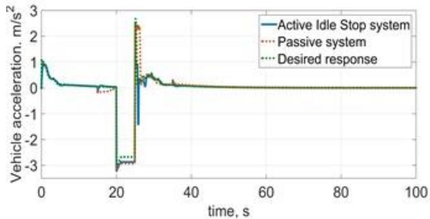
(a) Vehicle acceleration against time at 15 degree road gradient
