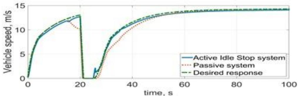
(c) Vehicle speed against time at 25 degree road gradient
