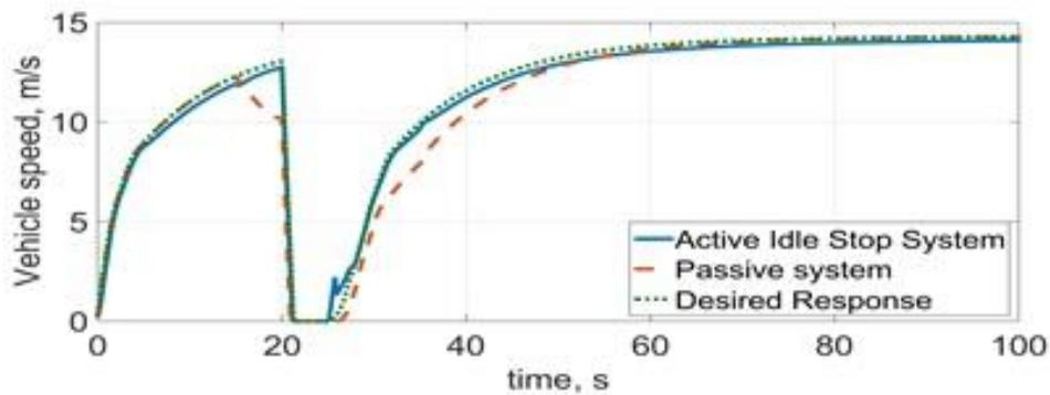
(a) Vehicle speed against time at 15 degree road gradient
