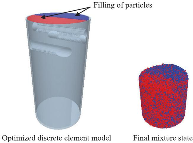
Figure 7: Mixture state obtained by the optimized discrete element model
