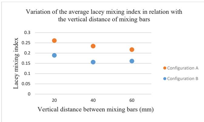
Figure 4: Variation of average mixing index in function of longitudinal distance between mixing bars
