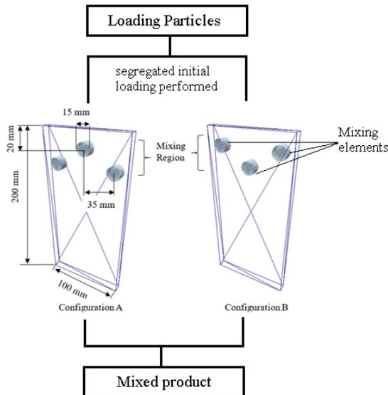
Figure 2: Mixing diagram including the geometry of the static mixer model setup with different configurations of mixing elements
