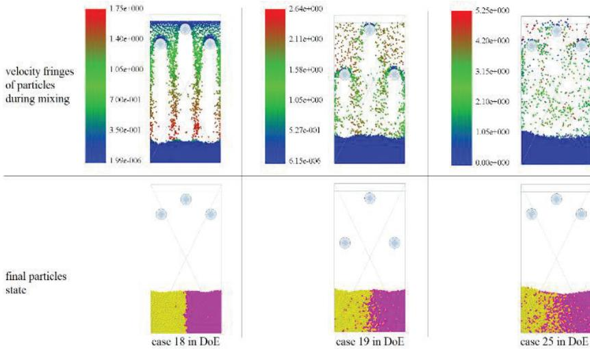
Figure 3: Velocity fringes of particles related to simulations 18, 19 and 25 in the DoE at  $t = t_{\text{mixing}}/2$  and their related mixture state at the end of the process
