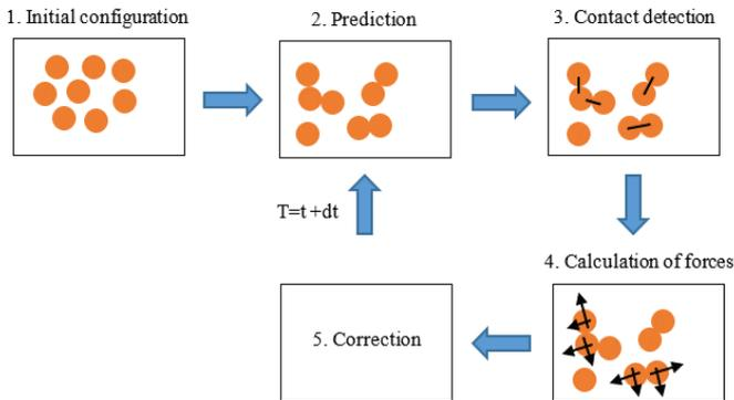
Figure 1: Description of the sequence steps of the discrete element method
