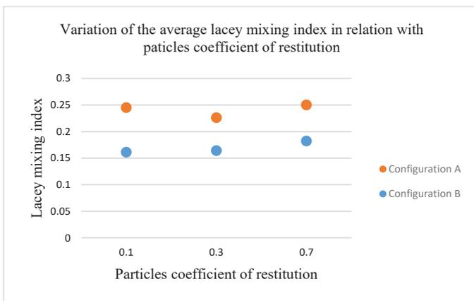
Figure 5: Variation of average mixing index in function of particles coefficient of restitution
