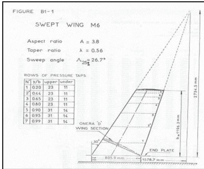
Figure 1: Layout of ONERA M6 Wing Planform [1]
