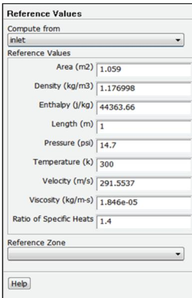
Figure 9: Reference Values Setting of the Wing Model
