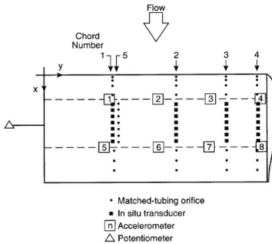
Figure 2: Instrumentation layout for the RSW model
