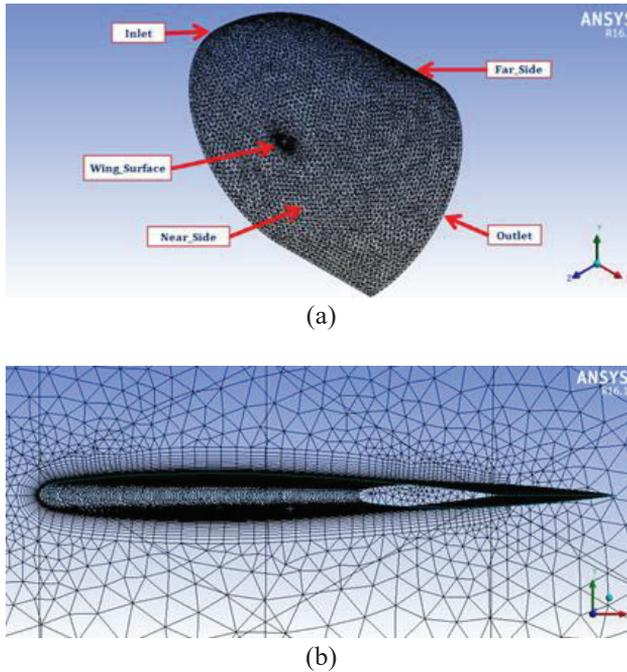
Figure 7: (a) Named Pressure Far-Field Boundary Condition; (b) Boundary Layer of ONERA M6 Wing
