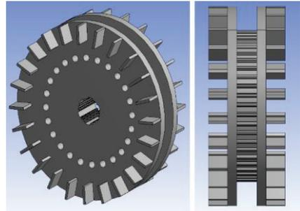
Figure 2: Modified Model of the Pulley
