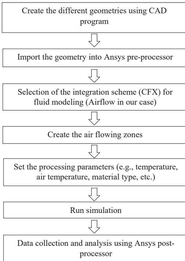
Figure 4: Schematic of the Finite Element Methodology
