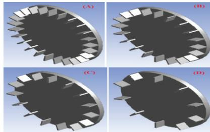
Figure 7: The modified models after adding the fins, Model (A) 25 fins, Model (B) 20 fins, Model (C) 15 fins, Model (D) 10 fins
