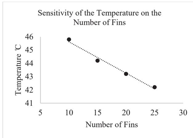
Figure 13: Sensitivity of the Temperature on the Fins Number
