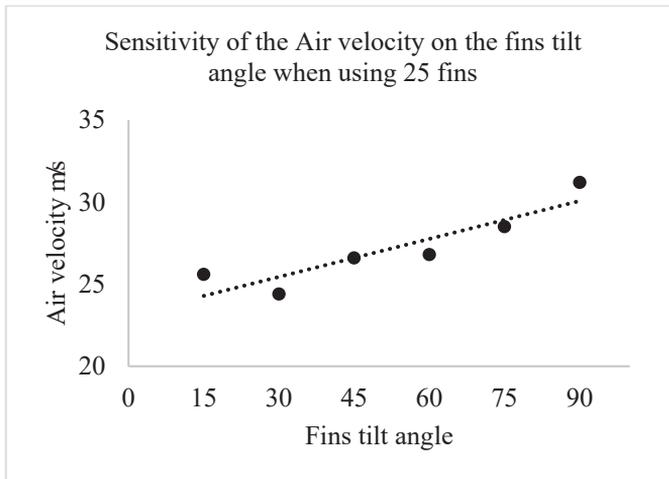
Figure 11: Sensitivity of the Air velocity on the fin orientation
