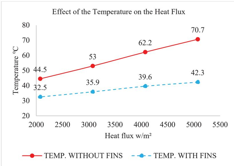
Figure 15: Sensitivity of the Temperature on the Heat Flux
