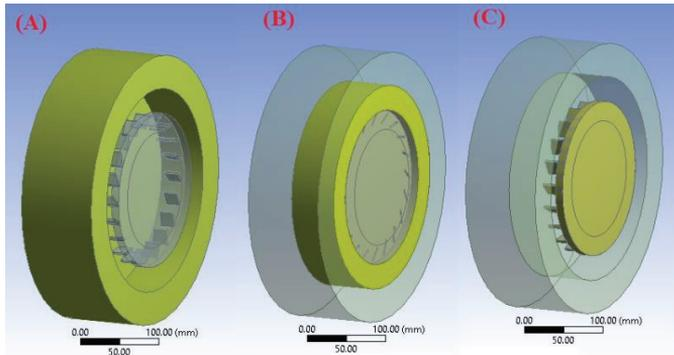
Figure 5: Different zones of the models (A) open air, (B) rotating air, (C) the pulley
