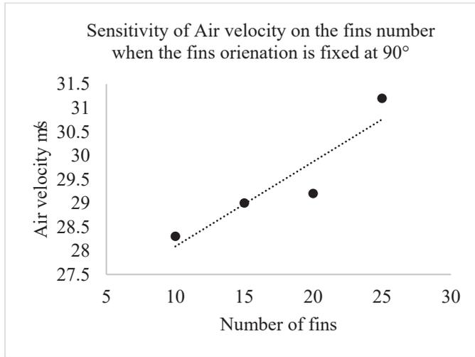
Figure 10: Sensitivity of the Air velocity on the fins number
