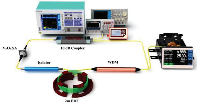
Figure 1: Schematic diagram of the experimental setup for the Q-switched EDFL with V<sub>2</sub>O<sub>5</sub> SA
