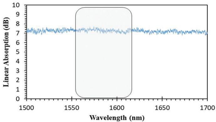
Figure 3: Linear saturable absorption curve for the V<sub>2</sub>O<sub>5</sub>-SA film
