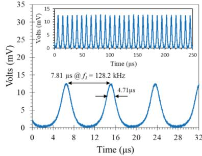
Figure 5: Typical pulse train of the Q-switched EDFL at 166.5 mW
