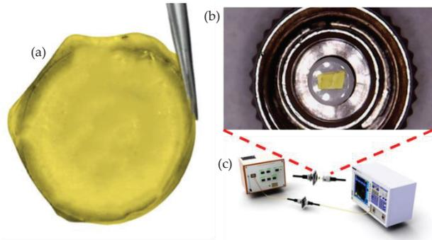
Figure 2: (a) A light yellow solid thin film of V<sub>2</sub>O<sub>5</sub> (b) the SA film placed onto a fiber ferrule tip (c) the linear saturable absorption measurement set-up
