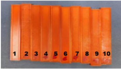
Figure 8: Printed test specimens of PLA material
