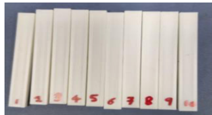
Figure 4: Printed test specimens of ABS material
