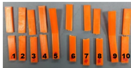
Figure 13: PLA specimens after the test
