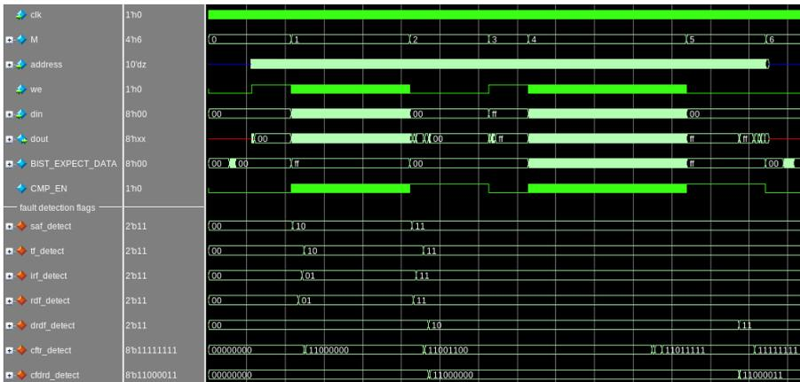
Figure 4: The March mSR fault detection simulation waveform
