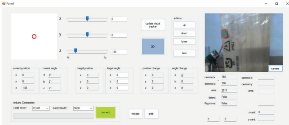
Figure 7: GUI layout of the Delta robot pick and place system
