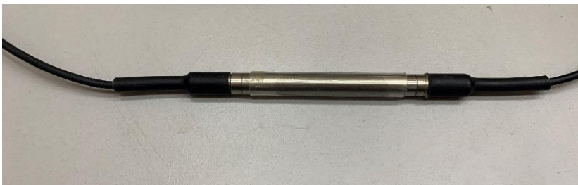
Figure 1: An Embedded FBG Temperature Sensor
