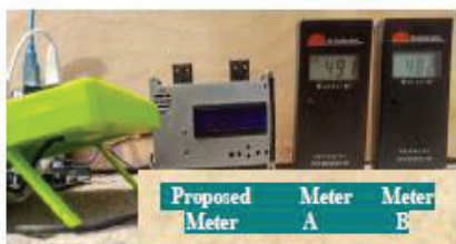
Figure 5: The proposed and two industrial daystar DS-05 pyranometers
