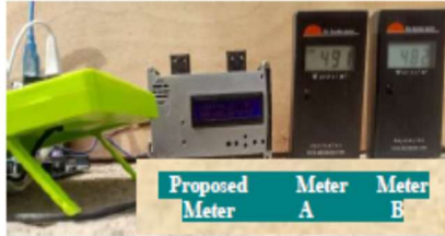
Figure 5: The proposed and two industrial daystar DS-05 pyranometers
