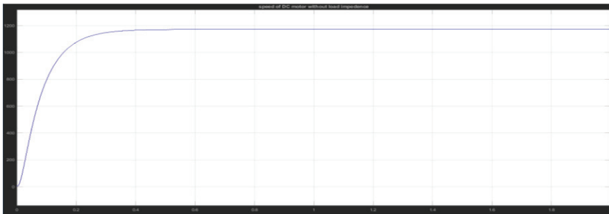
Figure 8: Speed of DC Motor Response when fed by Chopper Circuit with RC Filter
