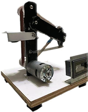
Figure 8: Completed mini sander machine
