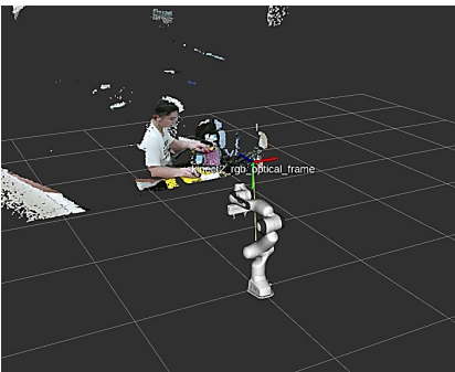
Figure 6: Alignment and transformation of the Kinect V2 with the environment in Rviz
