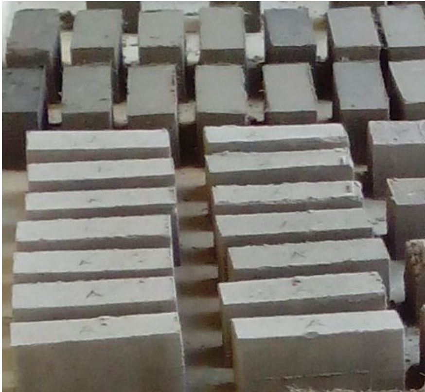
Figure 4. Lateritic bricks under curing
