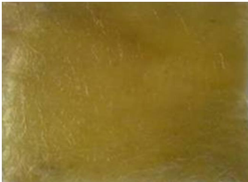
Figure 3. Hand lay-up composite sample before being cut into various standards
