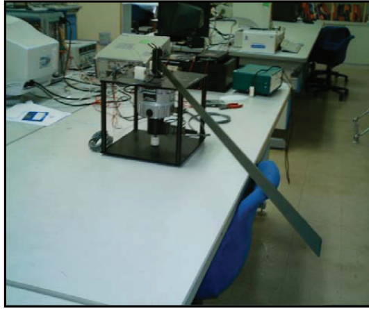
FIGURE 2 Experimental rig of the flexible manipulator system
