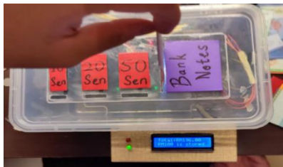
Figure 6: LCD Display Showing RM100 Stored
