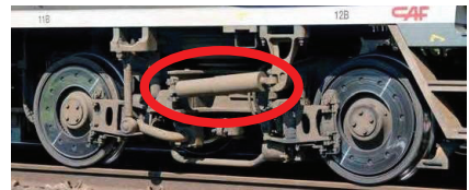
Figure 2: Secondary longitudinal damper [25]
