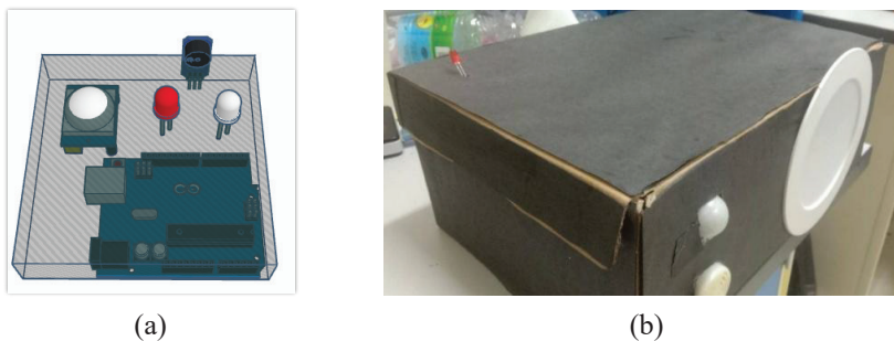
Figure 3: (a) The 3D Model of the Circuit Design, (b) Prototype Implementation of the Wild Animal Safety Fence
